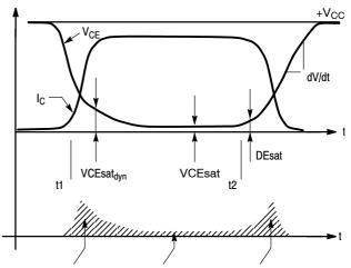
TURN ON LOSSES ON LOSSES TURN OFF LOSSES
