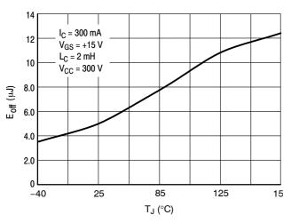
Figure 13. Switching Losses –E<sub>off</sub>– as a Function of Temperature
