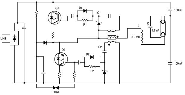
Figure 21. Self Oscillant, Low Cost CFL Basic Circuit
