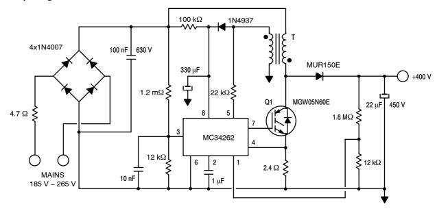
Figure 22. Basic Low Cost Power Factor Correction Circuit
