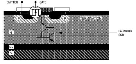
COLLECTOR Figure 7. Parasitic Thyristor into the IGBT Structure
