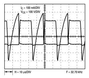
Figure 18. Steady State Operation (V<sub>line</sub> = 230 V)
