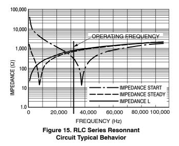
*Impedance START = impedance of the start-up network* built with the output inductor L and resonant capacitor C. Impedance steady = steady state impedance of the output inductor associated with the passive side of the half bridge. *Impedance L* = *impedance of the pure output inductor*.
