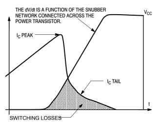
Figure 8. Switching Losses
