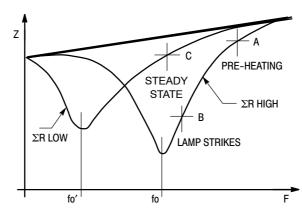
Figure 3. RLC Series Resonant Network Behavior
