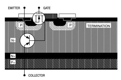
Figure 6. Typical Standard IGBT Die Cross Section
