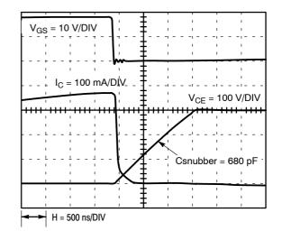
Figure 19. Switching Losses in the Steady State
