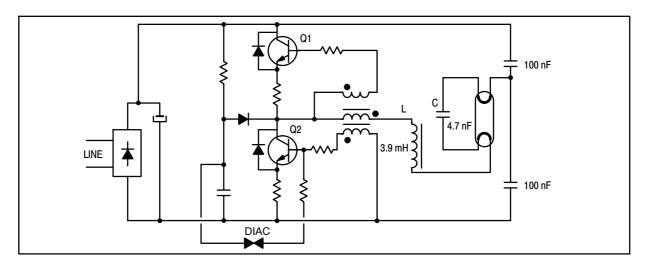
Figure 1. Basic Self Oscillant CFL
